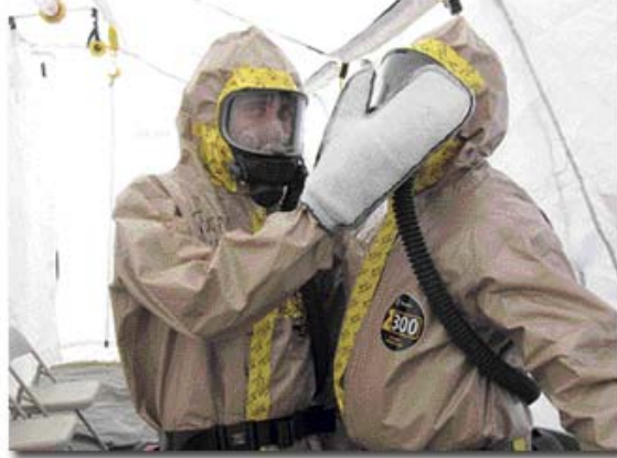
Fibertect® mitts can be used to decontaminate personal protective equipment. Photo courtesy of First Line Technology
